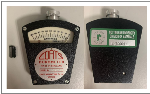
Figure 5. Durometer shore A hardness for evaluating the hardness of the seal.
