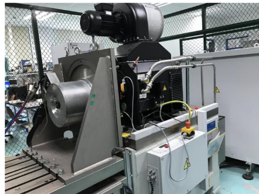
Fig. 1. Original 42kW 4-pole electrical machine
