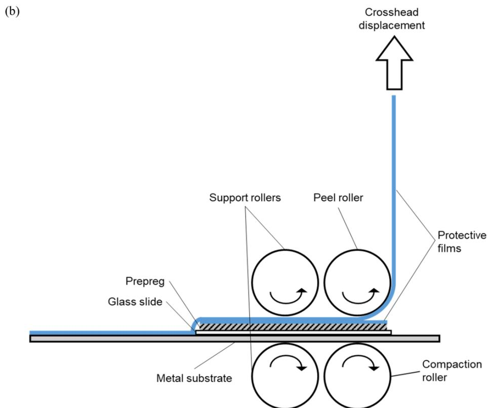
Fig. 2. (a) Specimen assembly for compacting the prepreg against the glass surface (the left edge is the leading edge of the assembly). (b) Schematic of the use of the tack testing fixture without the peel phase, enabling compaction only of the specimen assembly.
