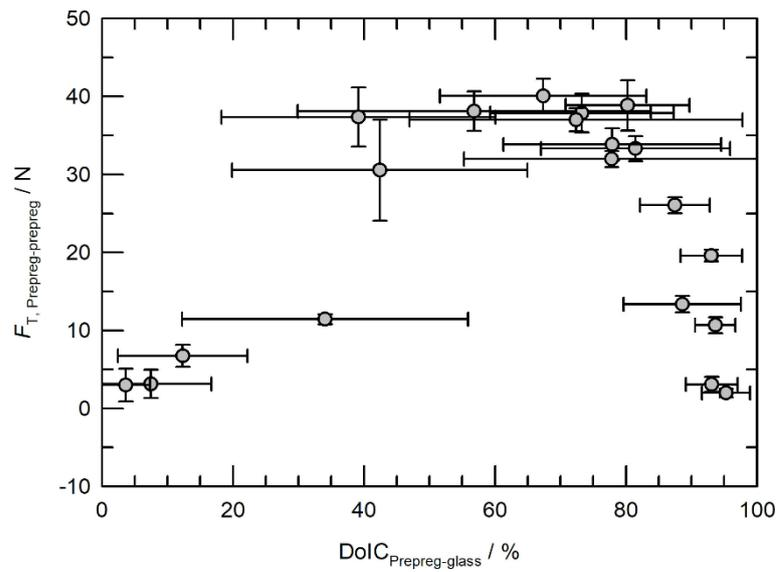
Fig. 9. Tack for prepreg-prepreg combination determined using the continuous application-and-peel test as a function of DoIC determined from prepreg-glass interface.
