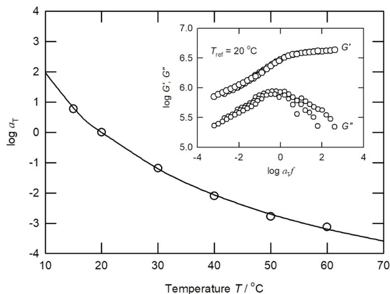
Fig. 4. Horizontal shift factors,  $a_T$ , obtained from the prepreg. The *solid line* indicates the Williams-Landel-Ferry equation (Eq. (1)). *Inset* shows the reduced frequency master curve of prepreg at  $T_{\text{ref}} = 20 \text{ }^\circ\text{C}$ .
