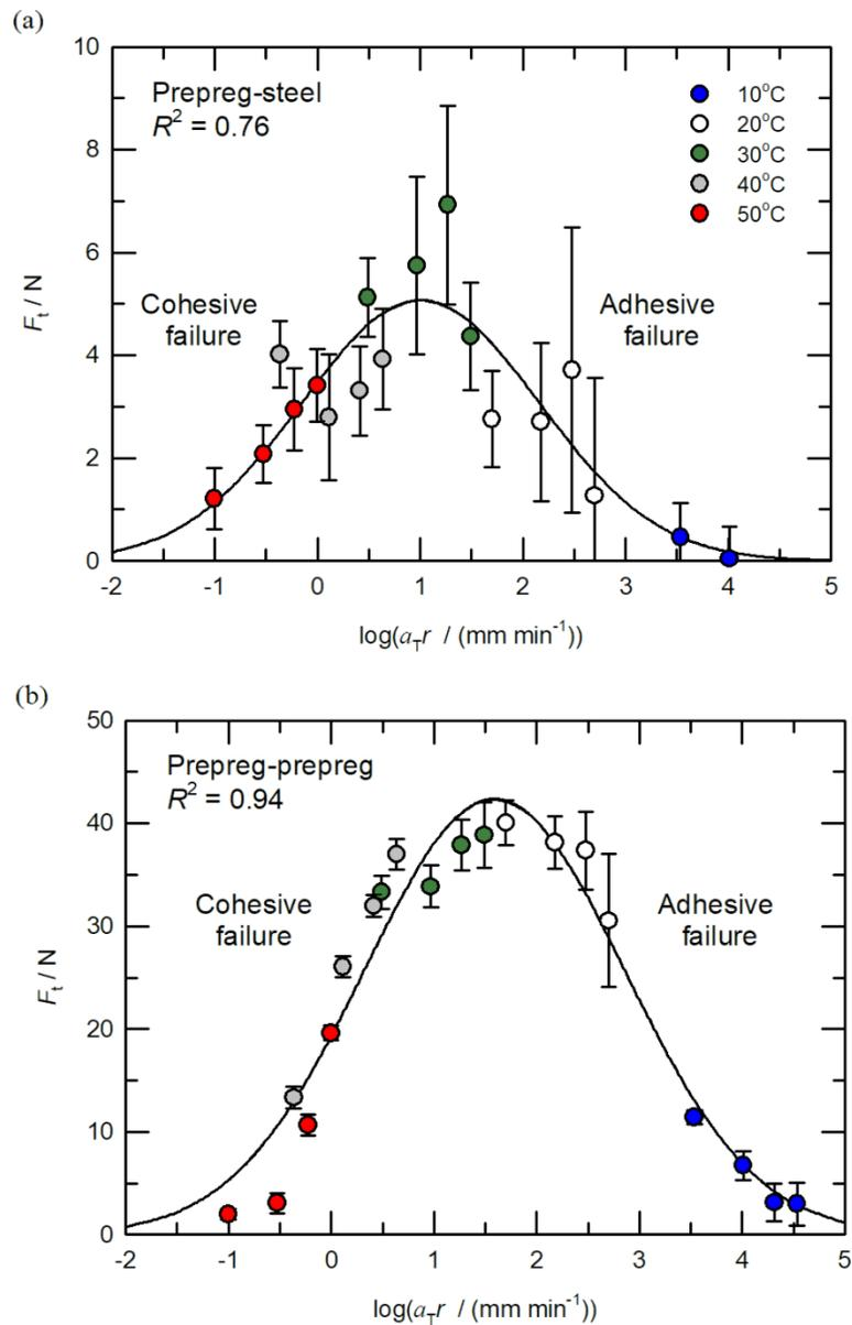
Fig. 5. Tack mastercurves for different surface pairings, based on data acquired at different temperatures,  $T$ , and feed rates,  $r$ , shifted to a reference temperature  $T_{\text{ref}} = 20^\circ\text{C}$ ; average values and standard deviations are indicated. The *solid lines* represent fits to Eq. (3) with the corresponding coefficients of determination,  $R^2$  shown.
