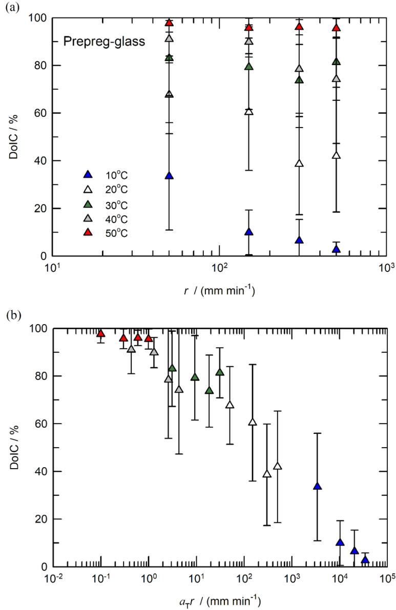
Fig. 7. (a) Degree of intimate contact, DoIC, for prepreg-glass pairing acquired at different temperatures,  $T$ , and feed rates,  $r$ ; average values and standard deviations are indicated. (b) The same DoIC data shifted to  $T_{ref} = 20$  °C using shift factors,  $a_T$ , determined from Eq. 1 (see Fig. 4).
