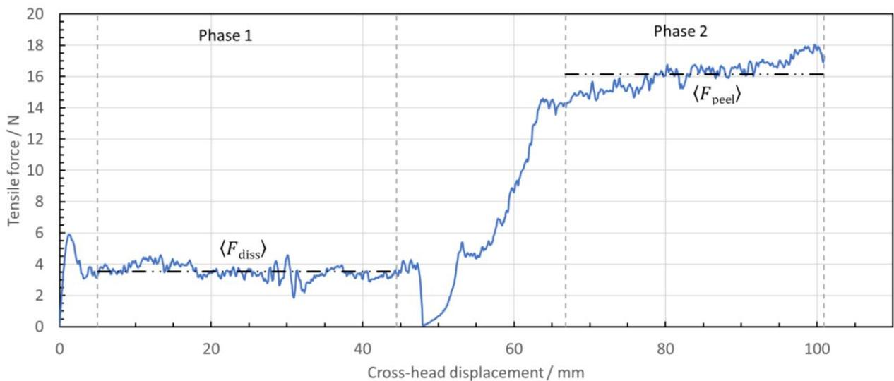
Fig. A1. Measured tensile force as a function of the cross-head displacement during a tack test for a surface combination of prepreg and steel at 40 °C and 50 mm min<sup>-1</sup>; the specimen width was 75 mm, and the compaction force 100 N. Vertical dashed lines represent the limits for the ranges used to determine the average force values (shown as horizontal dot dot dash lines) for each phase of the tack test.
