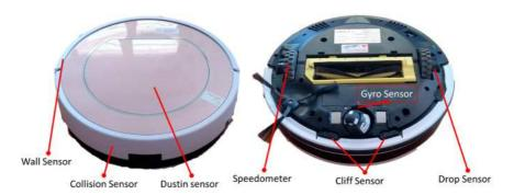
**Figure 8.2-1** The top and bottom view of an autonomous vacuum cleaner with internal sensors (gyro sensor, speedometer, suction sensor) and external sensors (dust-in sensor, cliff sensor, infrared sensor receiver, wall sensor, collision sensor, drop sensor).
