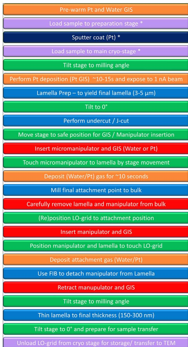
**Fig. 11.** Summary of the steps involved in performing a cryogenic Lift-Out, colour coded to highlight sample loading/unloading (lilac), platinum sputter coating (indigo), stage movements (green), GIS depositions (orange), manipulator movements and GIS insertions/retractions (red) and milling steps (blue). \*Sputter coating takes place in a preparation chamber if using Quorum system, if using other cryostages the location of sputtering and order of steps may vary.
