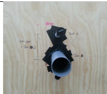
Testing plate B with three circular holes (two extended by pipes)
