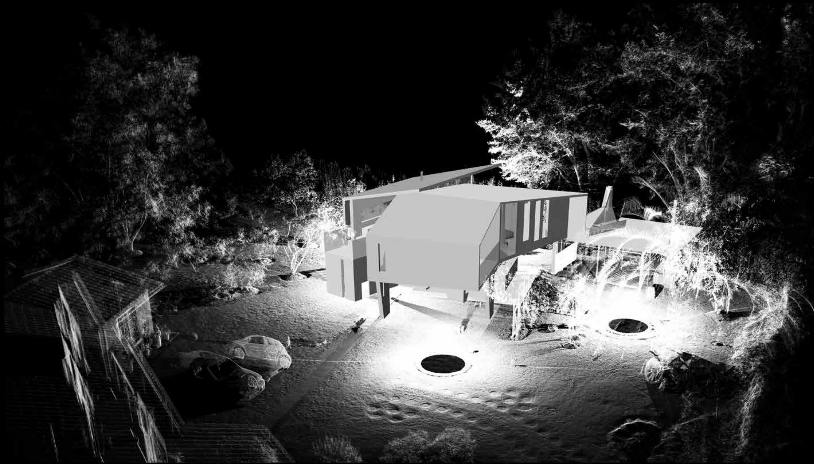
Figure 9. Aerial view of the design placed within the 3D laser scanning point-cloud, 2017. Source: B. Devilat & F. Lanuza.
