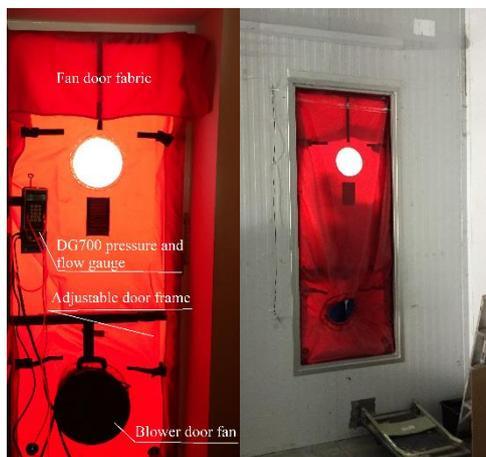
Figure 6 Setup of DBB in chamber 1 [40]
