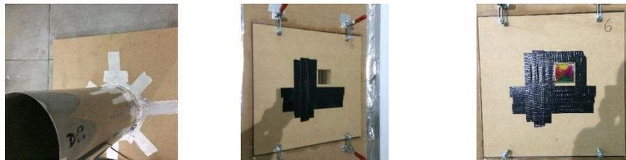
The individual testing plates were installed into the chamber envelope by means of an MDF panel sealed into a doorway. This MDF panel as shown in Figure 8, had a square opening with rubber gaskets installed along its edges. A testing plate could therefore be compressed against these gaskets to achieve an airtight installation. Four lateral press type clamps were used to compress the test plate against the gaskets to achieve easy, repeatable and airtight installation.
