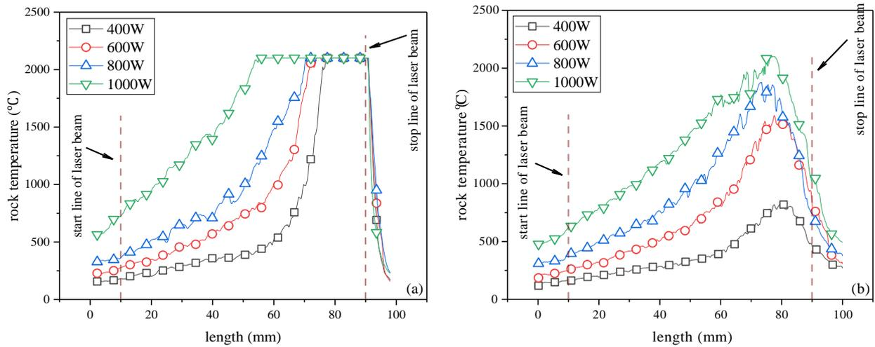
Fig. 4. Rock temperature distribution versus laser power (a) 160s (b) 200s.
