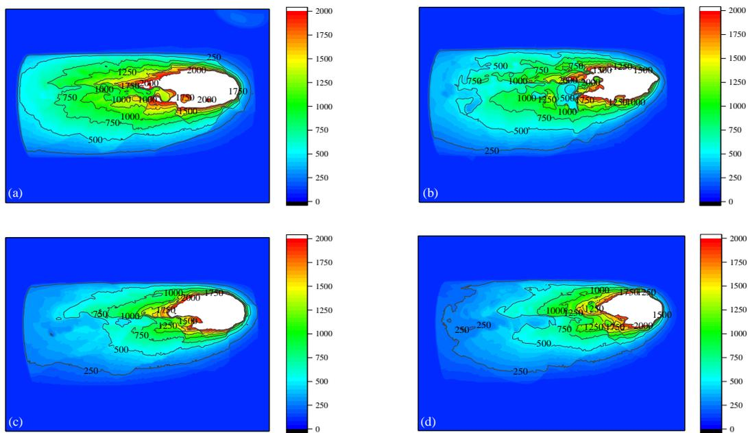
Fig. 5. Rock temperature versus beam diameter (a) 6mm (b) 8mm (c) 10mm (d) 12mm.
