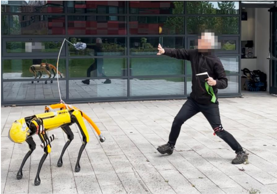
Figure 5. A 'whippy tail' with a soft weight on the end extended Spot's body and enabled more chaotic, playful collisions.
