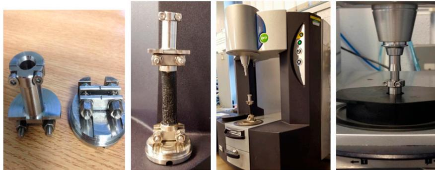
**Figure 2.** Mortar samples installation and test configuration.
