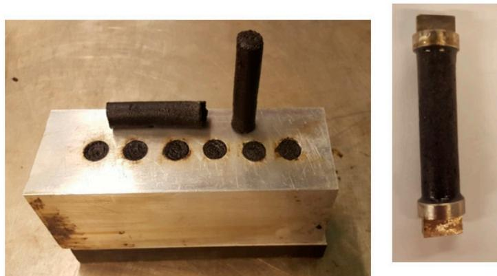
**Figure 1.** Steel mould and extracted mortar sample.
