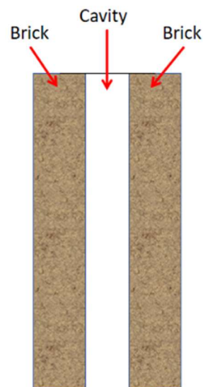
Figure 4. Double-layer cavity wall.
