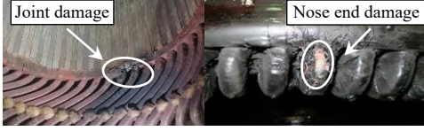
Fig. 19 Pictures of nose and joint damage
