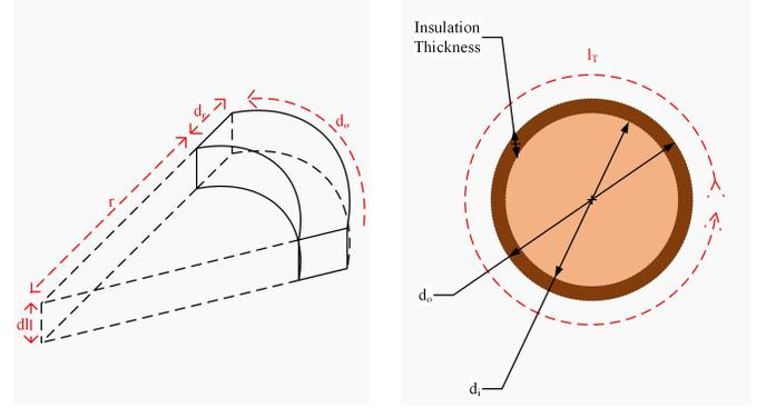
Fig. 6: Elementary Surface Turn-to-Turn Capacitance
