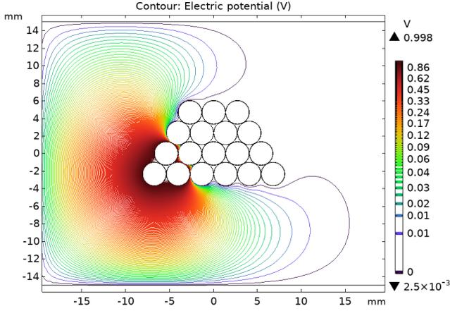
Fig. 9: Electric Field Trace in the Basic Cell
