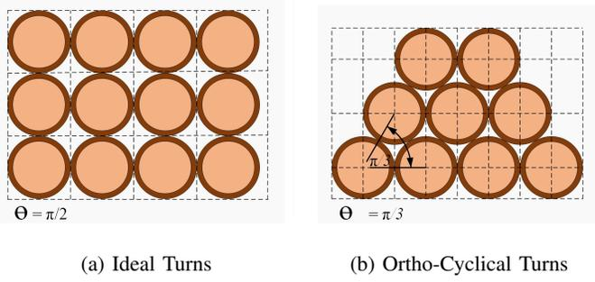
Fig. 1: Winding Arrangements for MLACs
