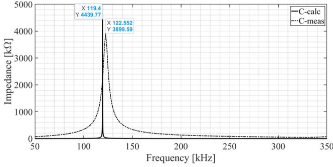
Fig. 12: Impedance Co-relation for the Prototype Inductor C
