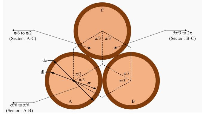
Fig. 2: Basic Cell's EFT Angles for an Ortho-Cyclical MLAC
