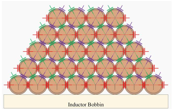
Fig. 4: Iterative Analytical Approach for the MLAC's Total Static Capacitance
