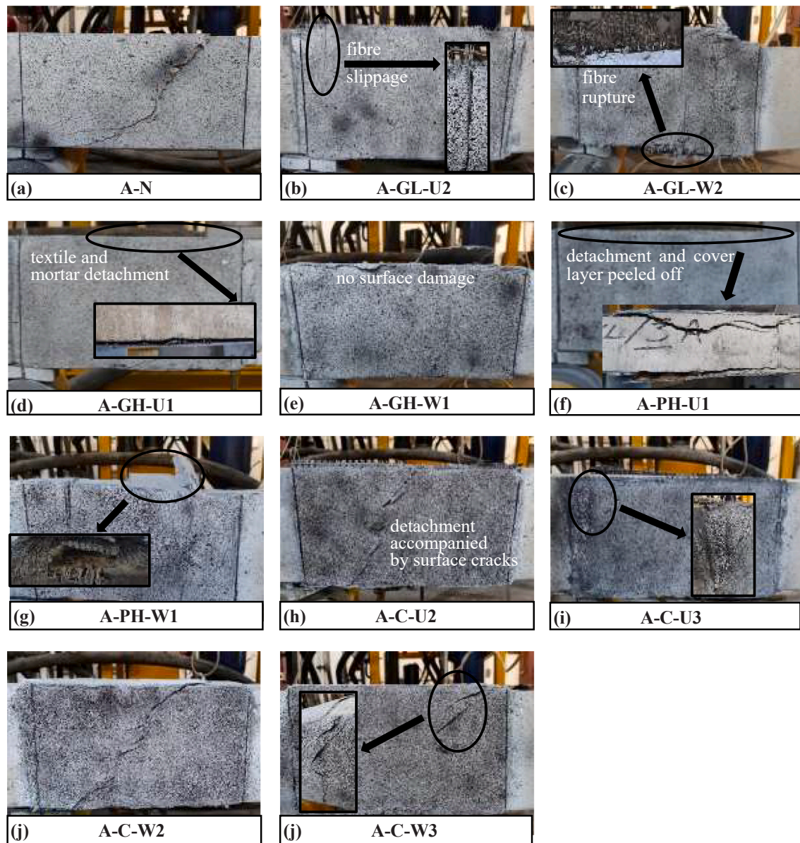
Fig. 5. Crack patterns and failure modes of Series A beams.
