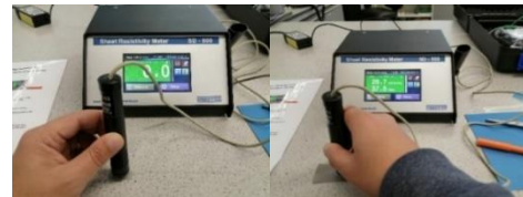
Fig. 8: Sheet resistivity measurement silicone-gel (Left), graphite (Right).
