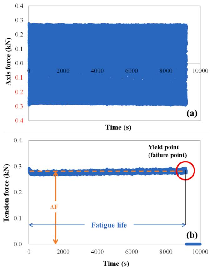
Fig. 5. (a) Raw data of the samples with brittle damage in the BF test and (b) the tensile force that the sample can withstand during the fatigue loading and the description of indicators in the case of brittle damage.
