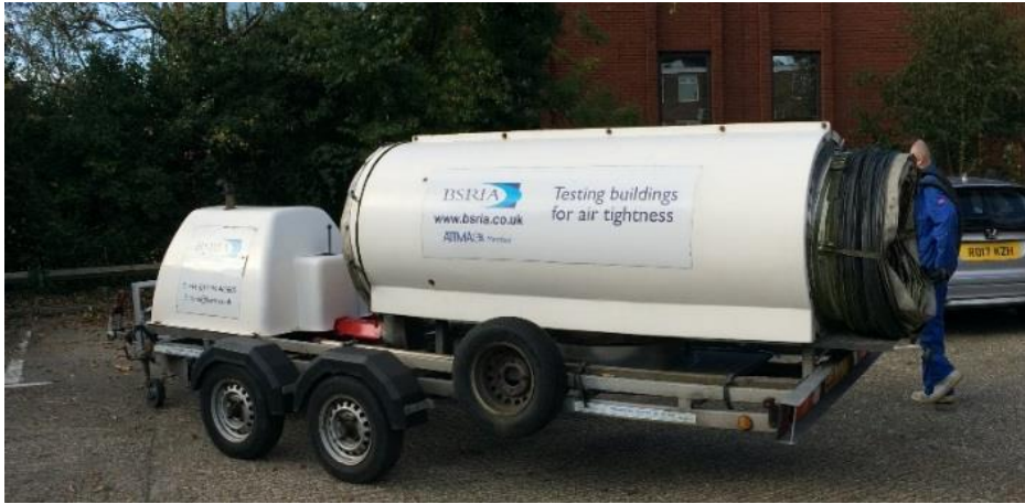
Figure 9 A petrol driven multi-gear portable trailer fan
