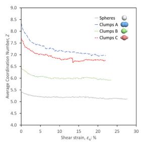
Fig. 6. Coordination number during triaxial shearing.
