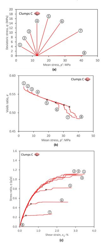
Fig. 9. Stress probes (a), volumetric responses (b) and deviatoric responses (c) for clumps C.
