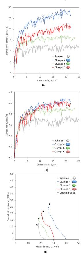
Fig. 5. Constant-volume triaxial results: deviatoric stress versus shear strain (a), stress ratio (b) and stress-paths (c).
