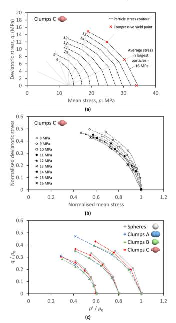
Fig. 10. Contours of average particle stress (a), and the same contours scaled and superimposed (b). Normalised contours for all materials (c).
