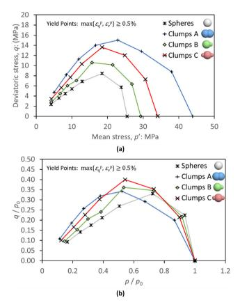
Fig. 11. Yield surfaces according to deviatoric and volumetric plastic strains.
