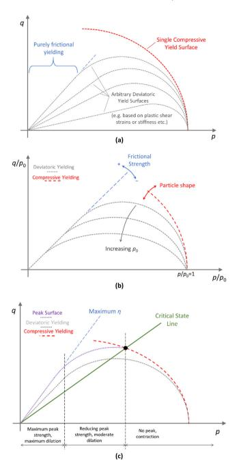
Fig. 12. Generalised yield surfaces: schematic showing frictional yielding, and general deviatoric and compressive yield surfaces (a); schematic showing effects of key parameters on yield surface shape (b); and general yield surfaces shown with respect to triaxial behaviour (c).
