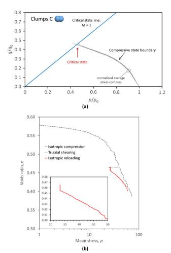
Fig. 13. Normalised compressive yield surface and critical state line for 11 clumps (a), and results for isotropically reloading sample after triaxial shearing (b).
