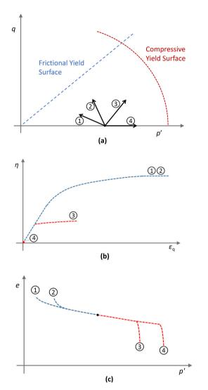
Fig. 8. Diagram showing idealised two modes of yielding: stress paths (a), deviatoric responses (b) and volumetric responses (c).
