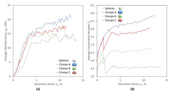
Fig. 4. Average particle stress (a) and average coordination number (b) as functions of volumetric strain.
