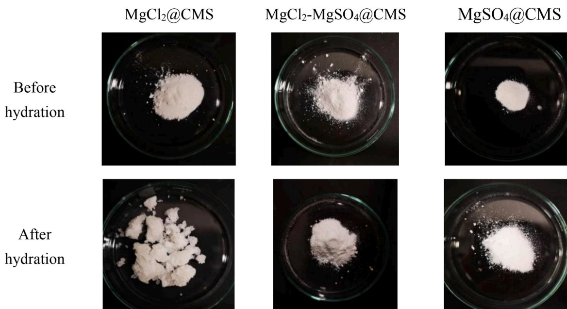
Fig. 9. Photos showing the appearances of the salt composite materials before hydration and after 10-h hydration at 60% RH, 30 °C, and 6 L/min.
