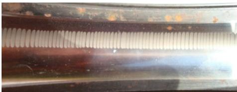
Figure 3: Damaged outer race of bearing due to bearing currents. [15]
