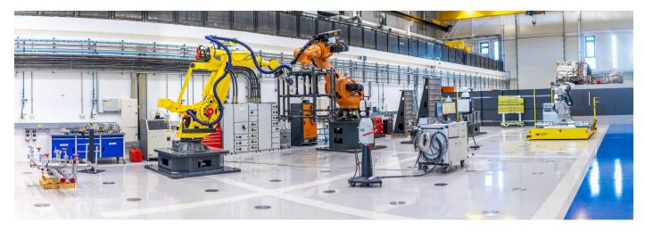
Figure 8: Omnifactory® - UK national training and research testbed for smart manufacturing system: Reconfigurable floor with calibrated floor points to locate robots within the facility
