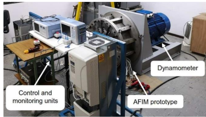
Fig. 14. Test bench and equipment used to operate the AF-MRIM prototype.
