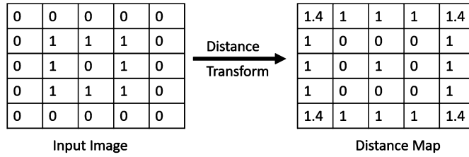
Fig. 2. Euclidean Distance Transform for a simple binary image: after applying the distance transform operator, the distance from each pixel to the nearest boundary pixel is calculated.
