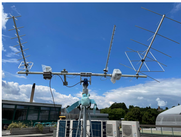
Figure 18. Tri-band ground station at the University of Nottingham during installation.
