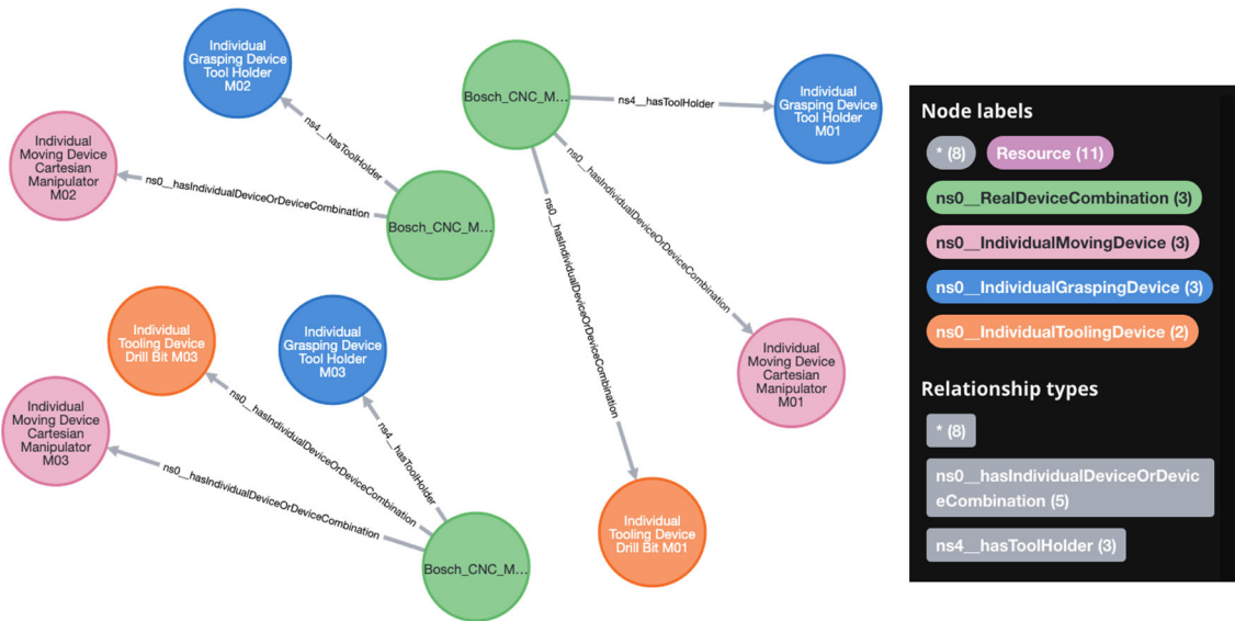
Fig. 6 Assets and related object properties that determine the assets’ capabilities as well as the similarity of concepts
