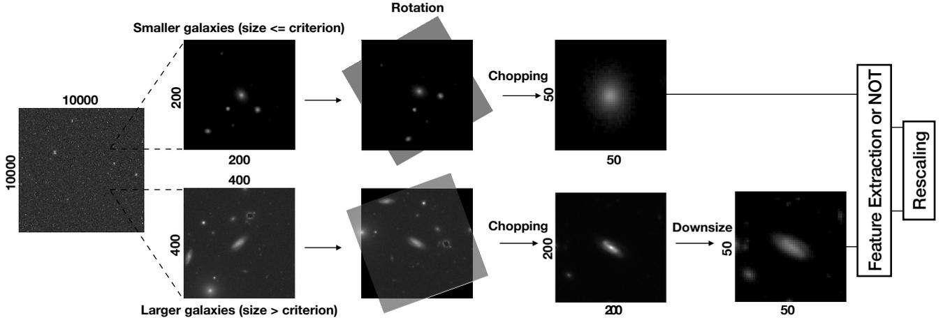
**Figure 1.** Pre-processing procedure pipeline. The pipeline starts from the initial coadd images, then we chop the coadd images into different sizes according to the size of galaxies. After rotation, we chop and downsize the images to the required sizes: 50 by 50 pixels. The details of the procedure is in Section 2.1
