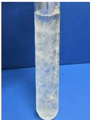
Figure 3: solution of 60.28wt% has serious phase separation at the first time melting
