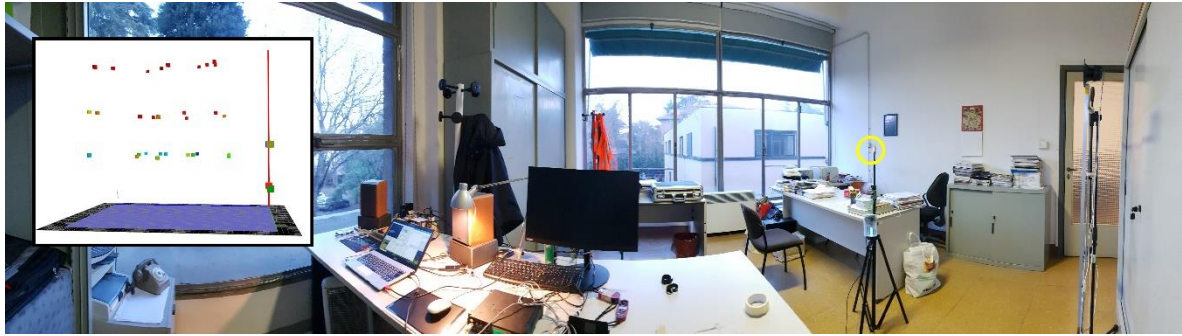
Figure 4: Panoramic view of the room being measured; in the box the measured points are visible in 3D.
