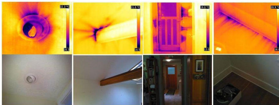
Figure 56: Thermal infrared images that show heat leakage from different parts of a house. Image taken from Ahomecheck, 2018
