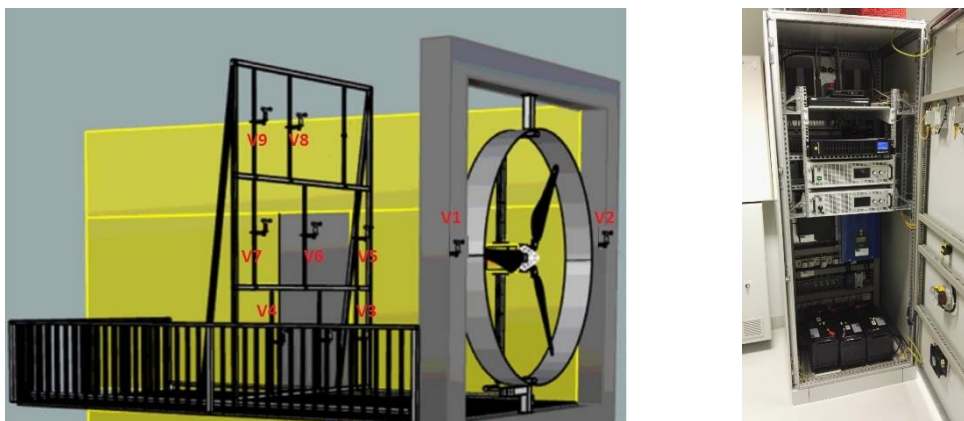
Figure 2: Visualisation of the anemometers location and the electric part of the experimental rig
