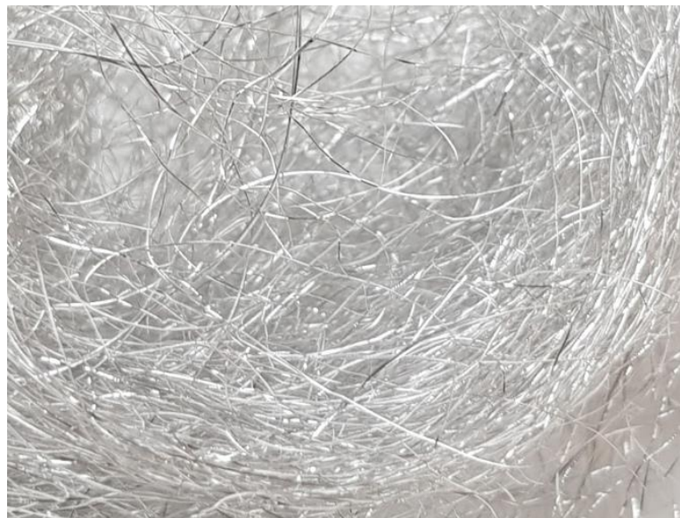
Figure 1: Close-up picture of the structure of aluminium wool
