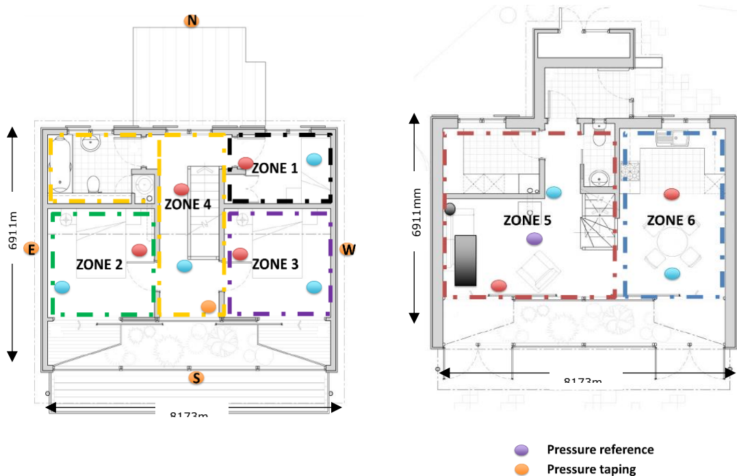
Figure 2. Top floor (left) and ground floor (right) of the test house; orange dots represent the places where the pressure tapings were allocated; the purple dot is where the pressure references was allocated, blue and red dots, represent a different experiment
