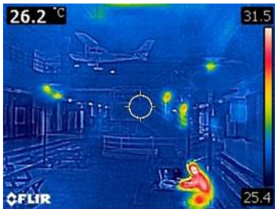
Figure 4a: Infrared thermogram showing heat sources in the department
