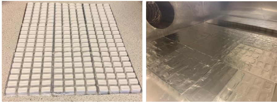
Figure 3: Left- set of 9 blister panels Right- panel testing in the control box.
