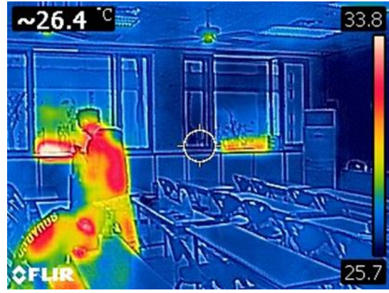
Figure 5b: Windows increase the temperature during the day
