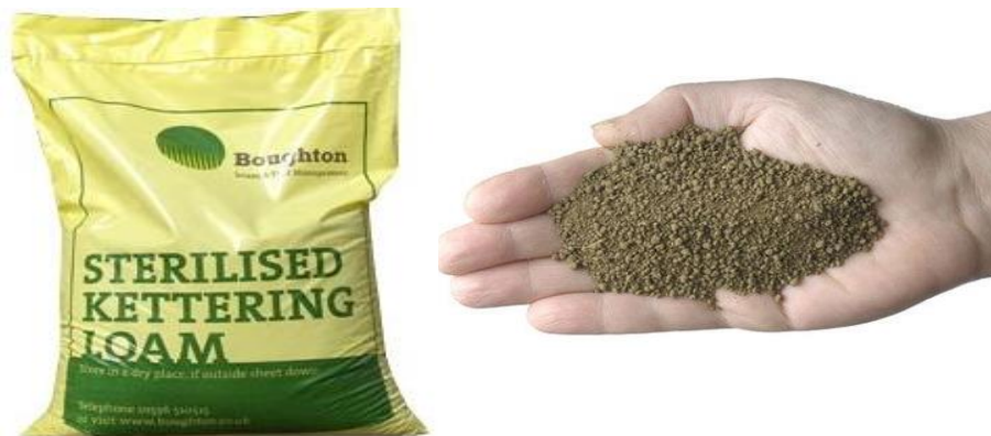
Figure 3: 25kg Bags of Dry Soil - Sterilised Loam that was used to fill the tank as the soil sample
