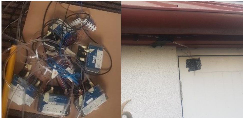
Figure 4. Differential pressure transducers used, one for each façade and one at the highest indoor point and; North pressure tapping.
