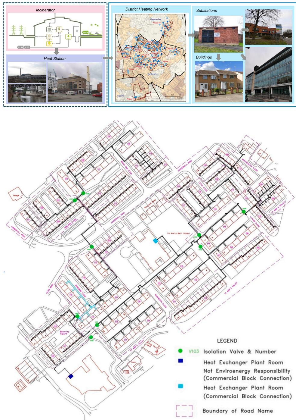
Fig. 8. (a) Heat generation and distribution across the Nottingham district heating network, and (b) pipeline of the district heating network in Phase 1 region.
