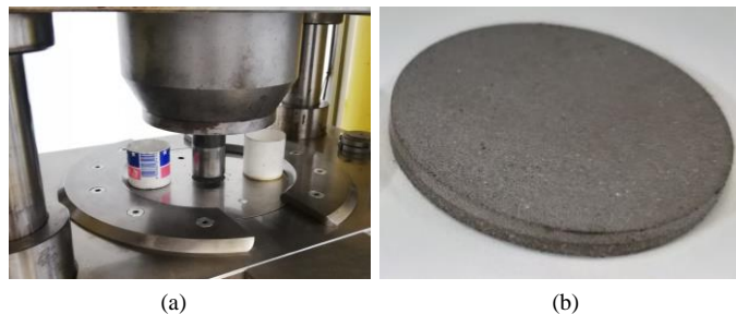
Fig. 2: Preparing multilayer magnet specimens, (a): hydraulic compression molding machine, (b): sample of a multilayer magnet (b).
