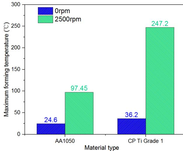
Fig. 3. The maximum forming temperature of AA1050 and CP Ti Grade 1 at different spindle speeds.
