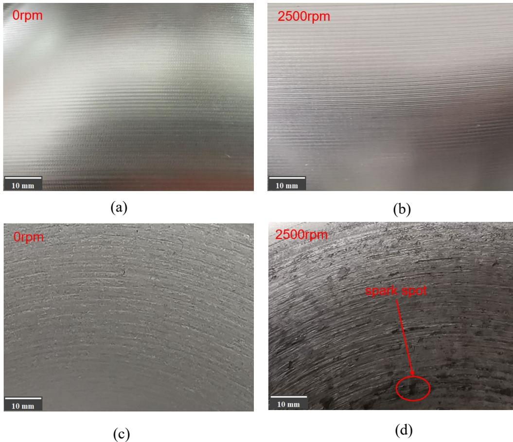
Fig. 5. The surface finish of formed part for (a) AA1050 at 0 rpm (b) AA1050 at 2500 rpm (c) CP Ti Grade 1 at 0 rpm and (d) CP Ti Grade 1 at 2500 rpm.
