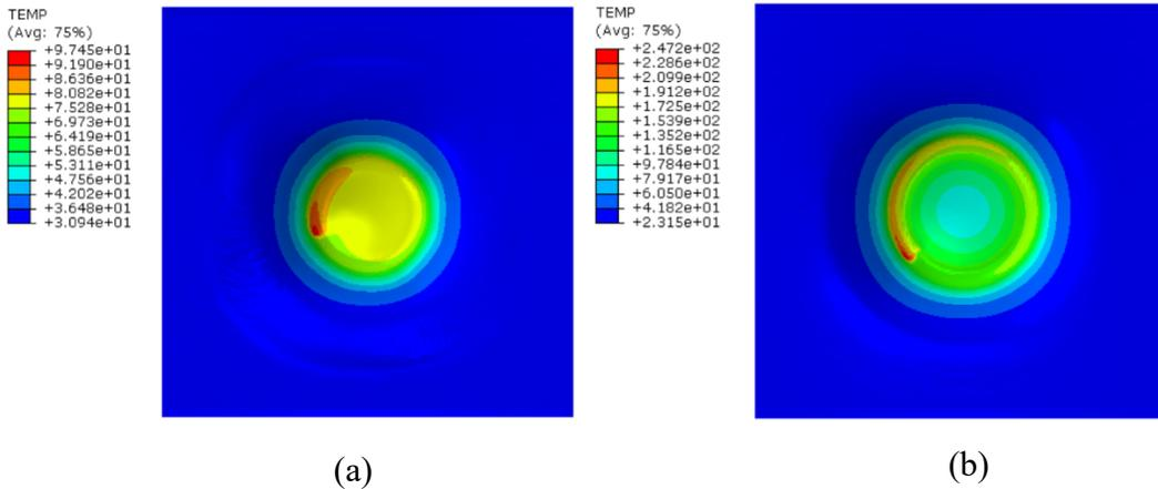
Fig. 7. The temperature distribution in the final stage of process with spindle speed of 2500 rpm for (a) AA1050 and (b) CP Ti Grade 1.
