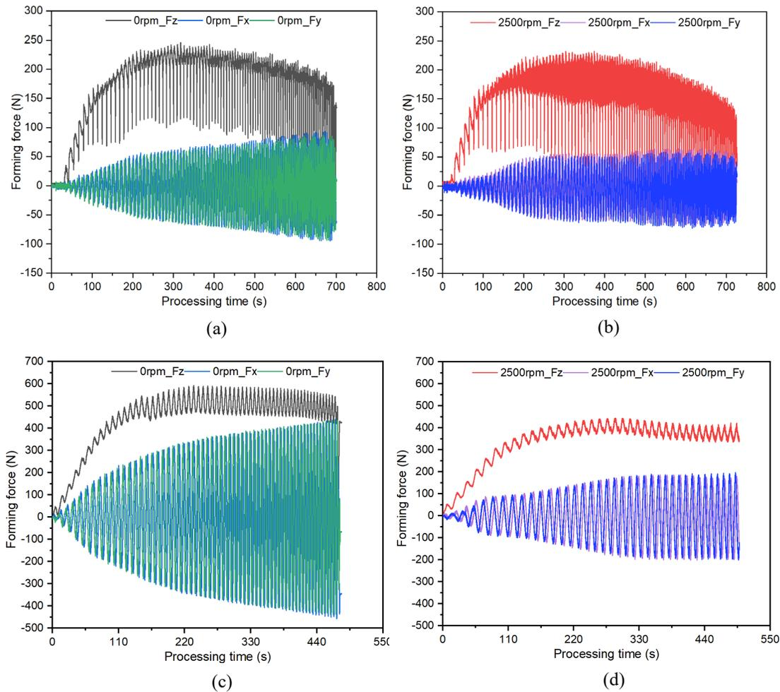
*Fig. 2. The variation of forming forces for (a) AA1050 at 0 rpm (b) AA1050 at 2500 rpm (c) CP Ti Grade 1 at 0 rpm and (d) CP Ti Grade 1 at 2500 rpm.*
