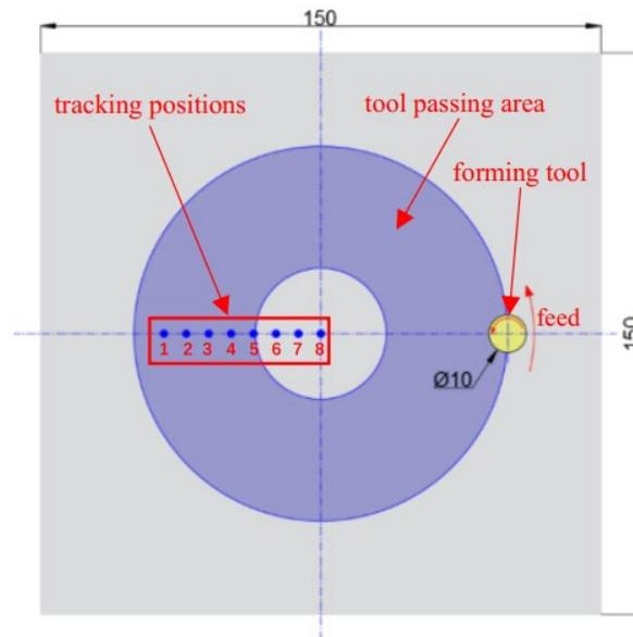
Fig. 1. FSIF tool rotation, movement and thermocouple tracking positions (unit: mm).
