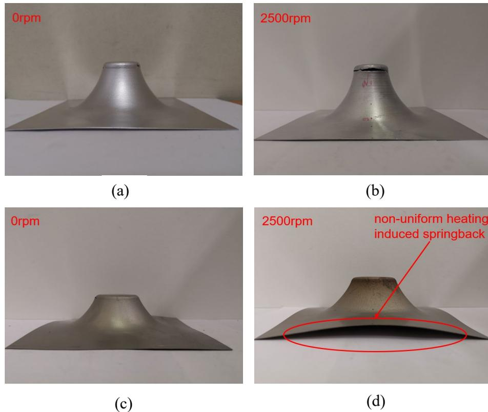
Fig. 4. The geometry of formed part for (a) AA1050 at 0 rpm (b) AA1050 at 2500 rpm (c) CP Ti Grade 1 at 0 rpm and (d) CP Ti Grade 1 at 2500 rpm.
