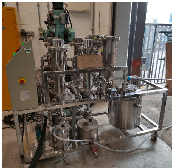
Fig. 1. Pyrolysis unit for production of rejuvenators.
