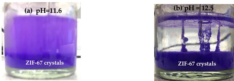
Fig. S27 Separation of ZIF-67 crystals from reaction solution for 10 min at -0.8 V at solution pH of a. 11.6 and b. 12.5.
