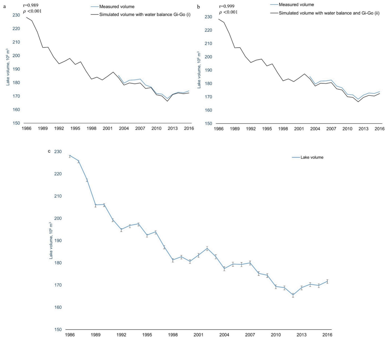
Fig 4. Model validation for Shortandy Lake. (a) volume simulated by the regional groundwater model, (b) volume simulated by groundwater flux estimated by water balance approach, and (c) water volume dynamics estimated by Eq 1, where errors bars show standard deviation of the lake volume obtained from a one-by-one sensitivity analysis with four selected model parameters.
