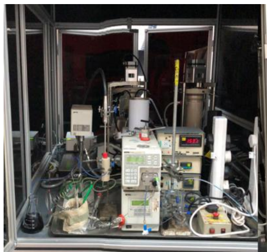
Fig. S6: Top – schematic of the larger scale telescoped photochemical and thermal reactions. Bottom – photographs of the actual equipment with the smaller vortex reactor. Note that the photochemical and thermal reactor assemblies and associated pumps are housed in completely separate vented cabinets with the reaction mixture pumped between them to ensure the safest possible operation in the presence of gaseous oxygen,.
