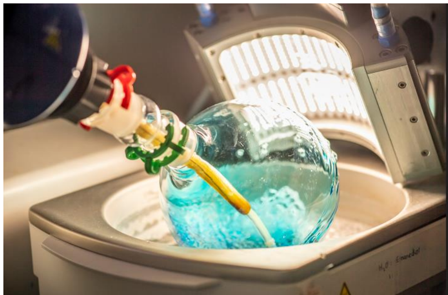
Fig. S1: General view of the PhotoVap with a 1 litre flask and a White LED assembly (Asynt Ltd) showing the tubes for filling and emptying the flask in the semi-continuous mode.
