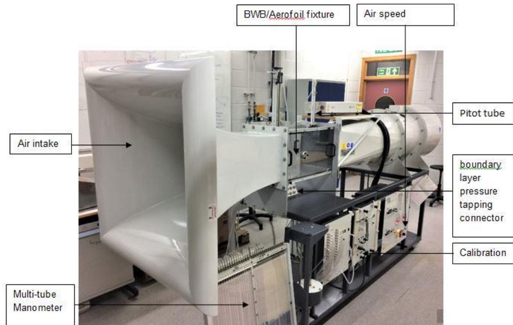
Figure 17. An open loop low speed wind tunnel that was used for testing the BWB model
