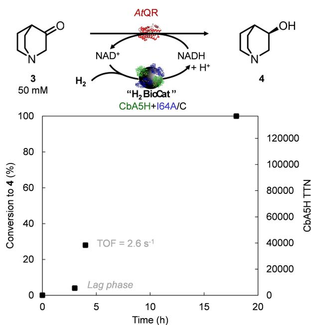
**Figure 5.** Biocatalytic hydrogenation of 3-quinuclidinone (**3**, 50 mM) to 3-quinuclidinol (**4**) using NAD<sup>+</sup> (1 mM), "H<sub>2</sub>BioCat" (CbA5H + I64A/C, 0.6 mg/mL) and AtQR (1.0 mg/mL) in Tris-HCl (50 mM, pH 8.0) under H<sub>2</sub> (1 bar) at 30 °C. 100% conversion was determined after 18 hours, which corresponds with CbA5H total turnover number (TTN) of 135,300. Turnover frequency ("TOF" = mmol<sub>4</sub> per mmol<sub>CbA5H</sub> per second) was calculated at 4 hours.
