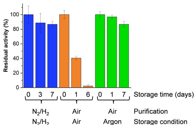
**Figure 3.** Characterization of retained activity of CbA5H over 7 days at room temperature, comparing purification and storage atmospheres. All values are mean values ± standard deviations from three independent measurements of H<sub>2</sub> evolution activity.
