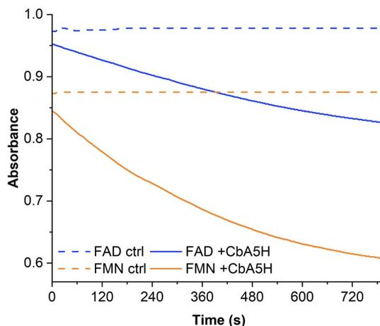
**Figure 4.** H<sub>2</sub>-driven flavin reduction by CbA5H. Reduction of flavins (0.1 mM aH<sub>2</sub> at 37 °C. FMN reduction was monitored at 445 nm. FAD reduction was monitored at 450 nm. The dashed lines show controls “ctrl” which were run in the absence of CbA5H.
