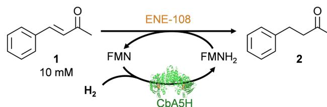
**Scheme 1.** Reduction of 1 to 2 using CbA5H (0.17 mg/mL), ENE-108 (0.5 mg/mL) and FMN (0.5 mM) in 10% v/v DMSO in Tris-HCl (50 mM, pH 8.0) at 35 °C under H<sub>2</sub> (1 bar). See S2.4 for more details.
