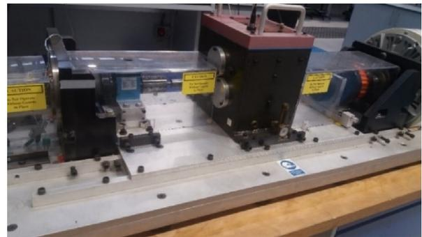
**FIGURE 7** The helicopter electro-mechanical actuation system test rig.
