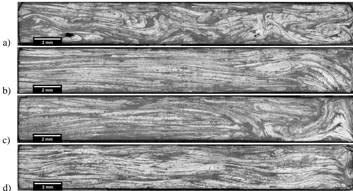
Figure 6: Micrographs (5x magnification) of the right hand edge, end of flow, for 40% (a), 60% (b), 80% (c) and 100% (d) mould coverages. All images are parallel to the flow direction
