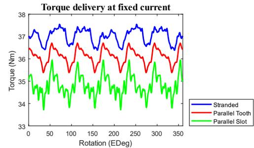
Fig. 7. Torque for fixed current of 85A
