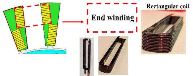
Fig. 4. Coil and end winding structures when using parallel tooth structure
