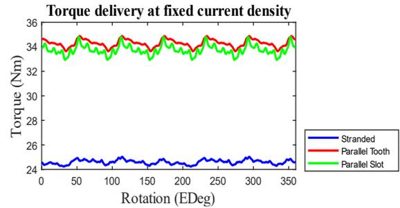
Fig. 6. Torque delivery per winding structure when operating at fixed current density 6A/mm<sup>2</sup>
