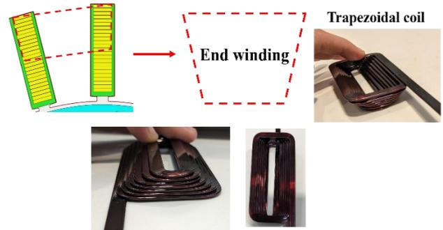
Fig. 3. Coil and end winding structures when using parallel slot structure
