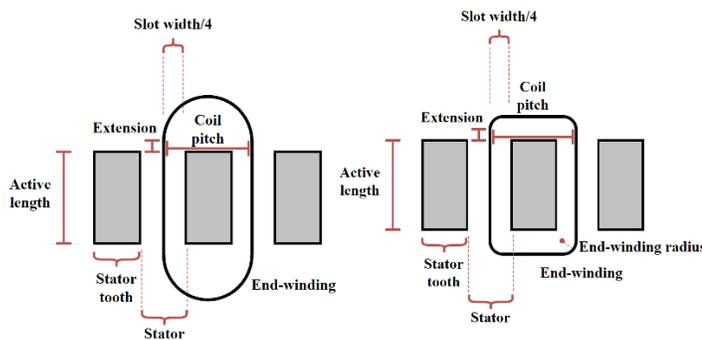
Fig. 5. Physical perspectives on manufactured coils
