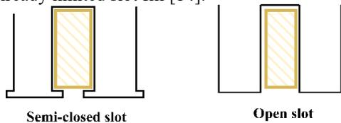
Fig. 2. Semi-closed slot structure and open slot structure
