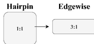
Fig. 1. Hairpin and edgewise winding aspect ratio difference
