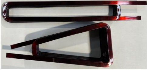
Fig 1. Illustration of coil windings manufactured using edgewise-insulated wires.
