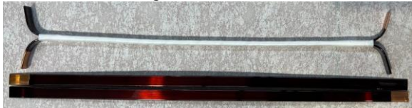
Fig. 2. Illustration of edgewise insulated wires shown both before (below) and after (top) being wrapped in PTFE, representing the test sample.
