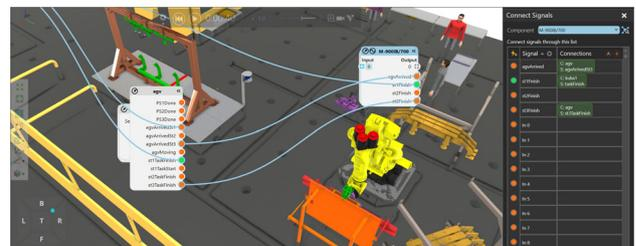
**Fig. 5** Communication among different components or agents (internal communication). The internal communication among different components is based on event-triggered communication. The signals are shown in the above figures with light blue solid lines
