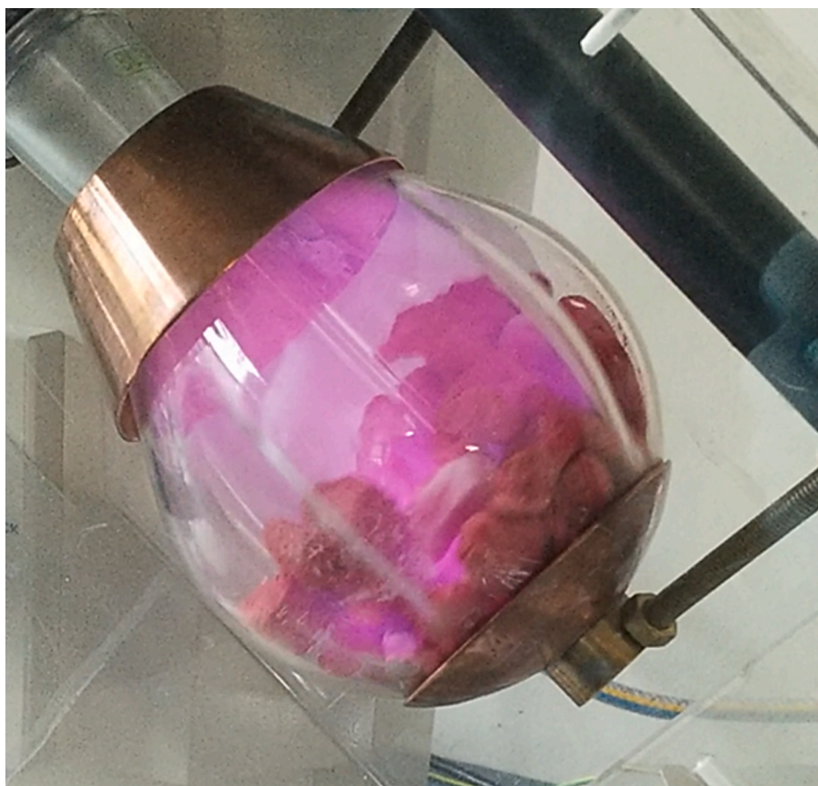
Fig. 1. Rotary Plasma reactor set-up from a modified rotary evaporator developed by Michl et al. (2015).
