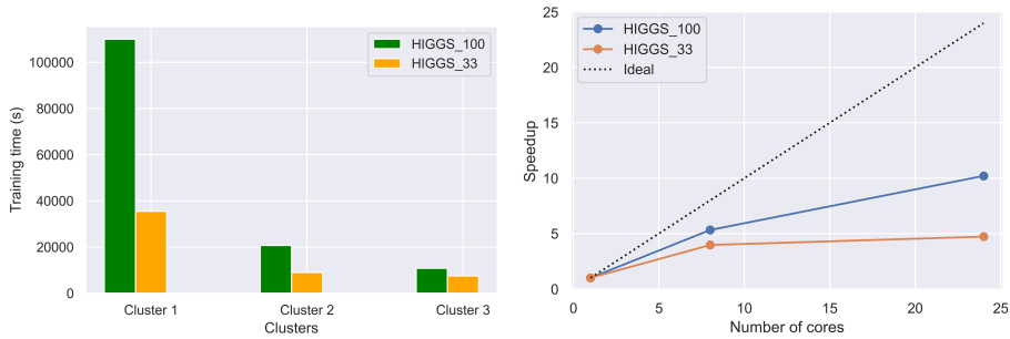
(a) Training time comparison between clusters in HIGGS dataset (b) Speedup comparison in HIGGS dataset
