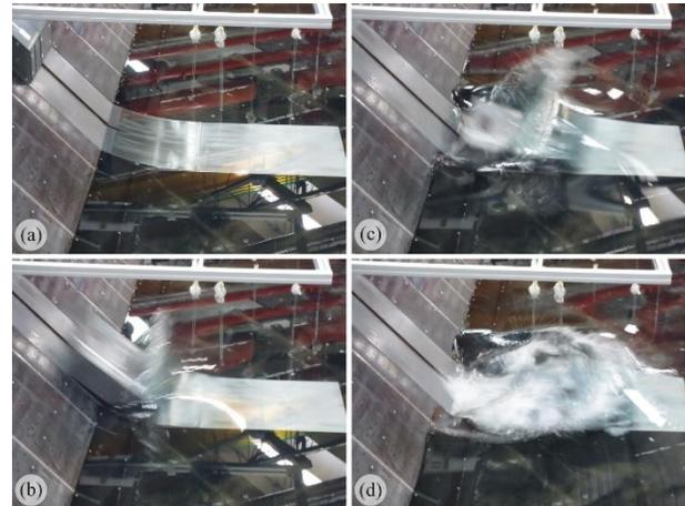
Figure 2 - Picture series of SLT generation in an idealised 3D laboratory experiment (Heller and Spinneken, 2015).
