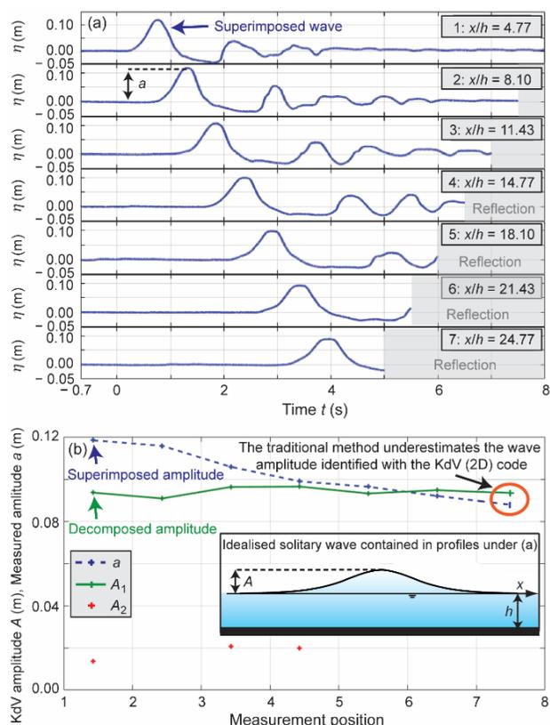
Figure 3 - (a) SLT profiles  $\eta$  (m) versus time  $t$  (s) measured at seven distances from the slide impact in a flume (2D) and (b) wave amplitudes  $a$  together with primary  $A_1$  and secondary solitary wave amplitudes  $A_2$  identified with the KdV (2D) method in the data in (a) (after Brühl and Becker, 2018).
