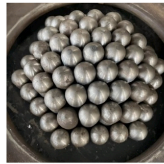
Fig. 7. Multi point die set-up for experimental testing.
