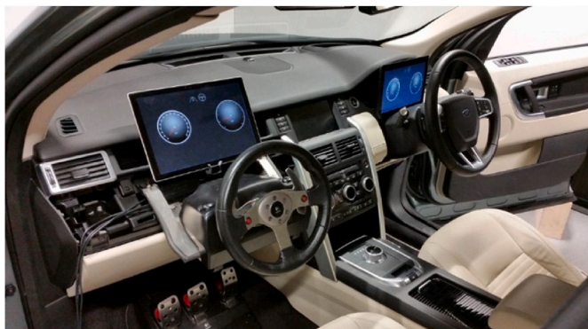
Fig. 1. Driving simulator set-up to simulate handover between two drivers.
