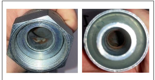
Fig. 4. Parts with rust identified within end fitting [15]
