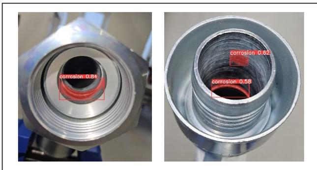
**Fig. 6.** Crimp Fittings after the image segmentation
