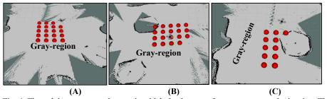
**Fig. 4.** The red dots represent the area in which the drone performs coverage path planning. The gray area represents a region in which the UAV is certain there is no obstacle, i.e., path-planning can be performed on it. The dark edges in the gray regions are obstacle or no-fly zones identified based on the principle of occupancy grid mapping, and the remaining part of the graph in light green represents the unexplored area.
